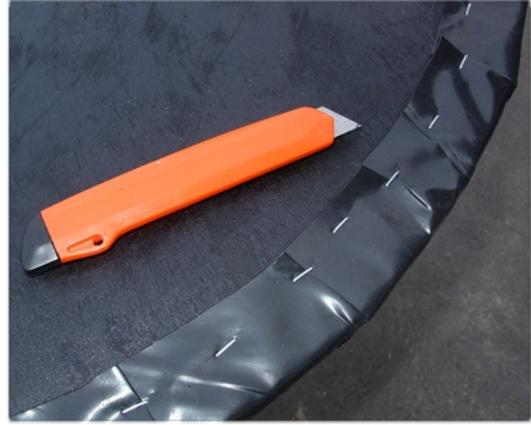
5. Lay the plywood disk on the center of the plastic sheet. Fold the edges of the sheet up over the plywood and staple it to the top of the plywood platform. Place a staple every 10 cm.
