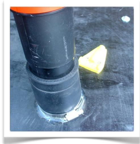
10. Turn the platform around and insert the PVC pipe into its hole. Glue it down with silicone and let dry. When dry, push the rubber connector onto the pipe and affix with the clamp.
