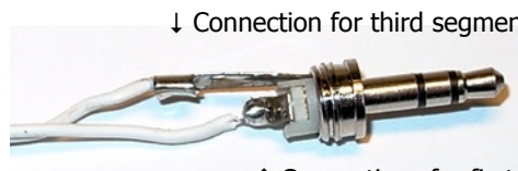
↑ Connections for first two segments of plug. Connect these to the POSITIVE of the flashlight batteries if used with an iPod Shuffle
